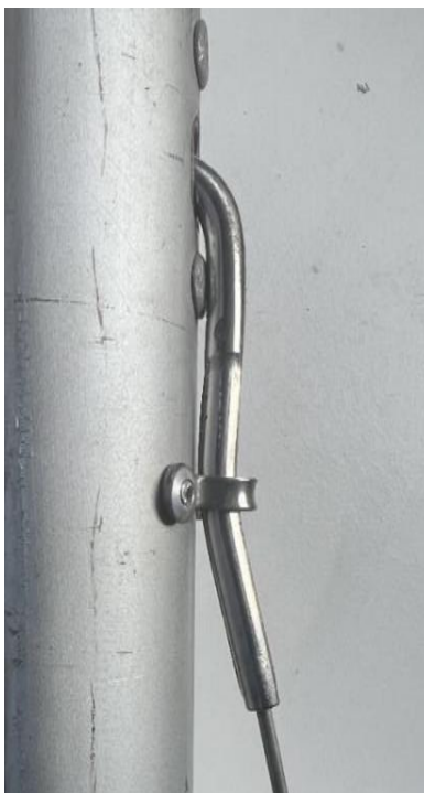
Fig 2. Forestay attached to the mast through a sheeve box modified by a saddle fitting.
